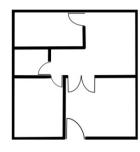
**Floor Plan:** a drawing that shows the view from directly above a building.
